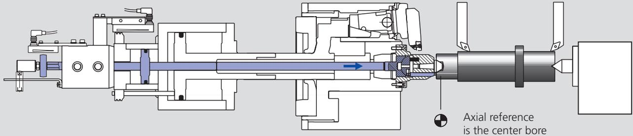
**Power operated face driver with fixed center type SNF
